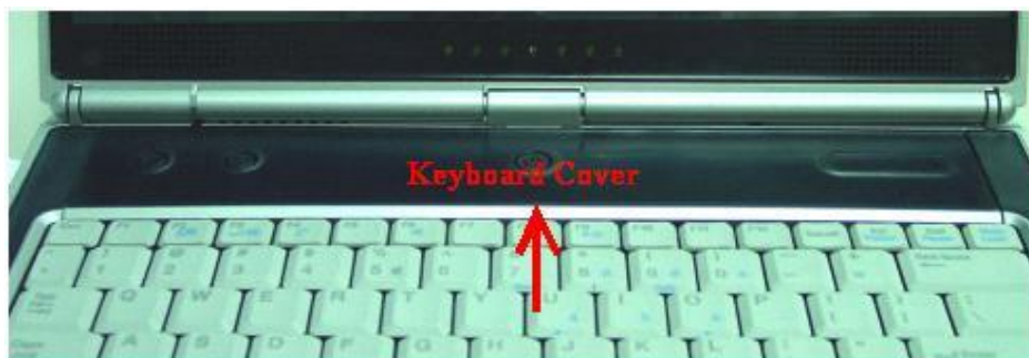
Figure 2-3 Remove keyboard Cover
