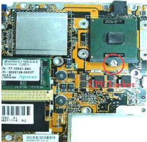
Figure 2-7 Remove CPU
