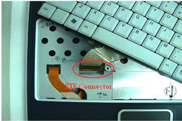
Figure 2-4 Remove keyboard
