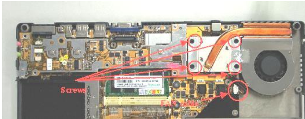
Figure 2-6 Remove heat sink plate and Fan
